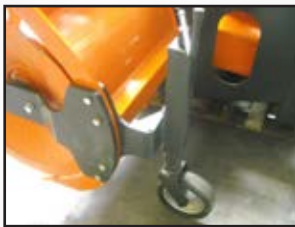
Ruote laterali pivotanti a 360°. Side slewing 360° free wheels.
