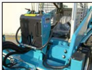
Supporto reclinabile del distributore. Reclining control valve support.
