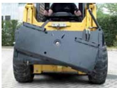
The Tilt-Tach connection system is an interface located between the Skid-Steer Loader linkage and the attachment. Thanks to its hydraulic right/left oscillation, the Tilt-Tach is the ideal tool to fix charge's level on rough grounds or for many other operations such as drainage ditches digging with the bucket corner. It's standard equipped with 2 rubber hoses with quick couplers kit and universal linkage plate.
