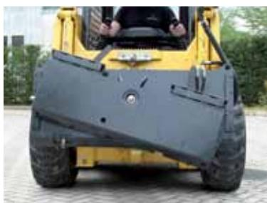
The Tilt-Tach connection system is an interface located between the Skid-Steer Loader linkage and the attachment. Thanks to its hydraulic right/left oscillation, the Tilt-Tach is the ideal tool to fix charge's level on rough grounds or for many other operations such as drainage ditches digging with the bucket corner. It's standard equipped with 2 rubber hoses with quick couplers kit and universal linkage plate.
